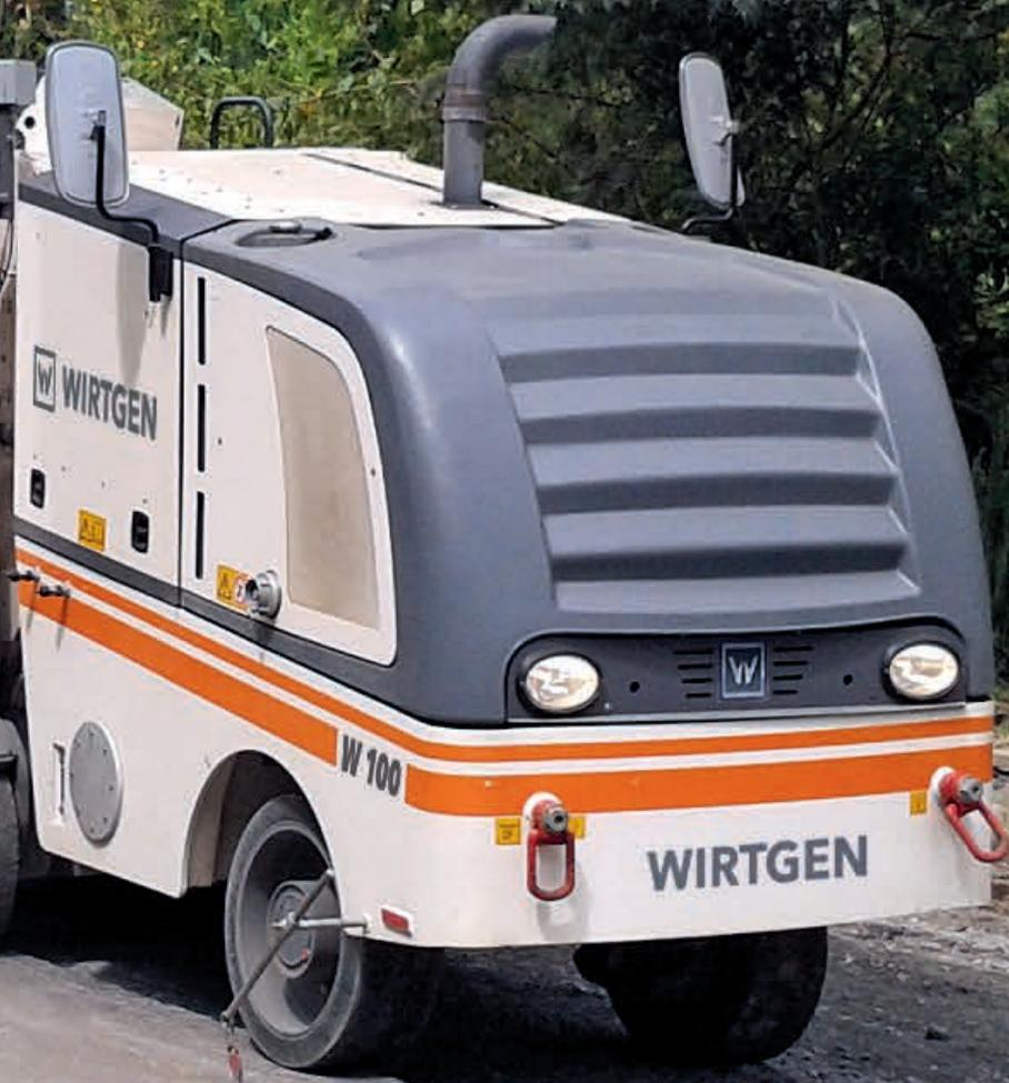
The manoeuvrable small milling machine is the ideal candidate for efficient milling operations in the one-metre class.
