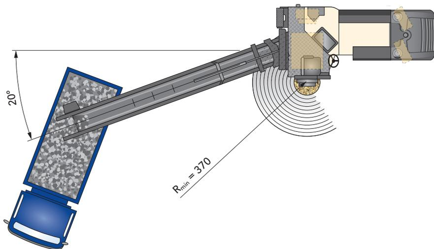
Milling radius, 50 mm milling depth, dimensions in mm
