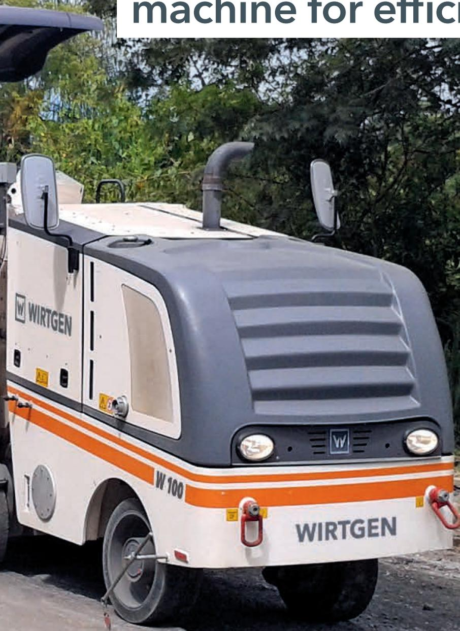
The manoeuvrable small milling machine is the ideal candidate for efficient milling operations in the one-metre class.
